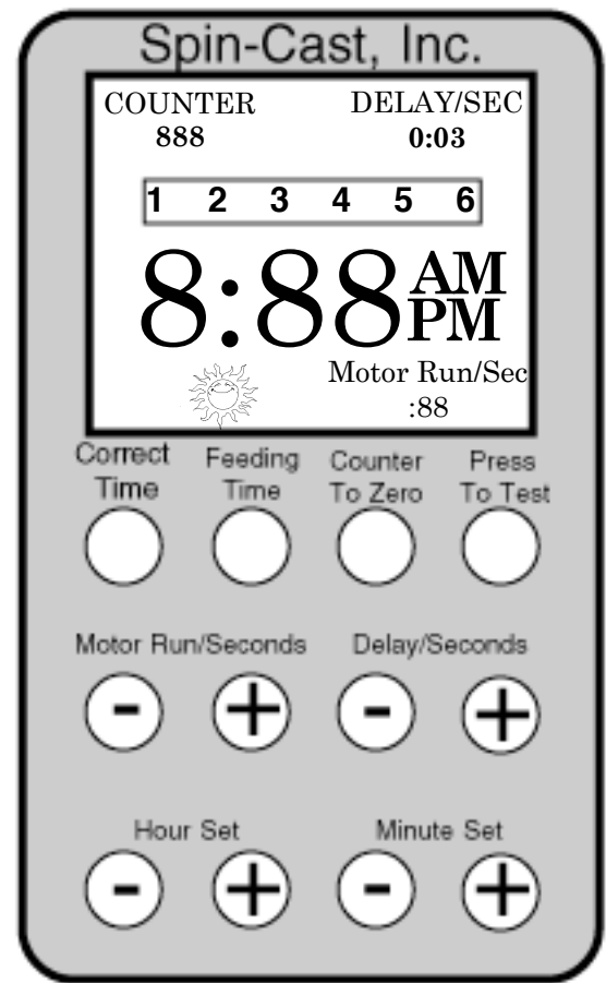
SCREEN DISPLAY DURING PRESS-TO-TEST OPERATION
